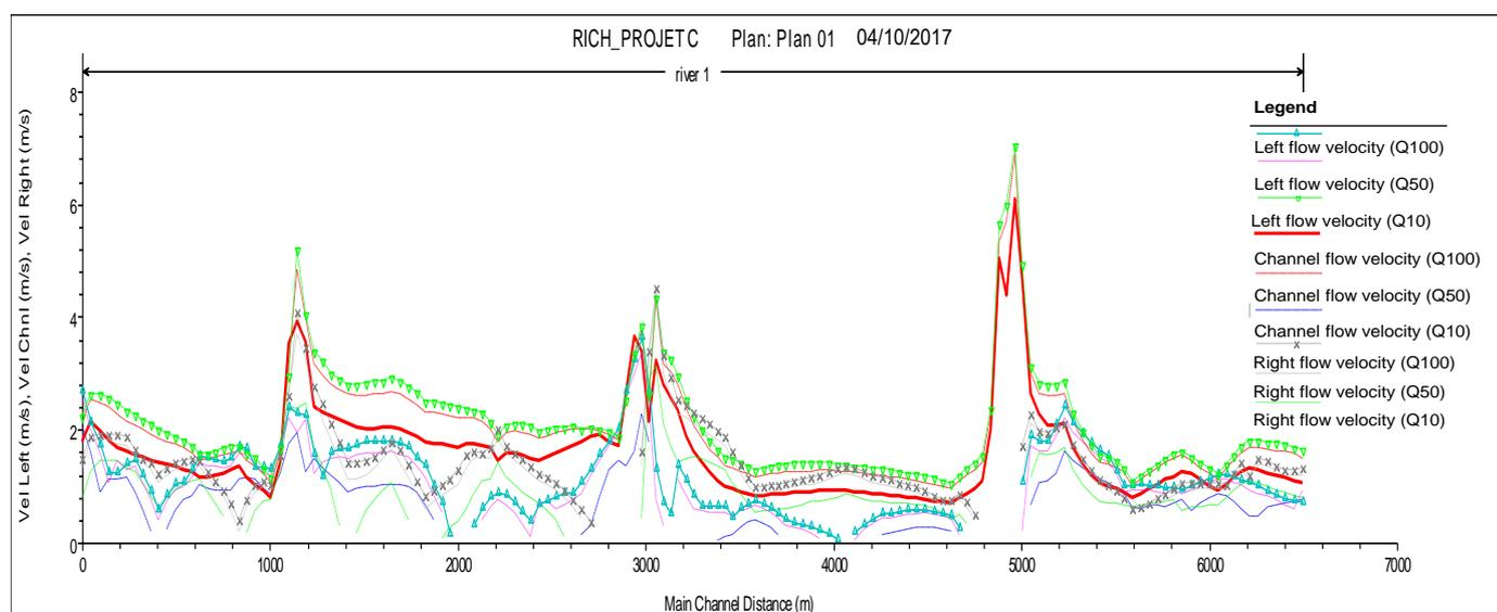
**Figure 13:** Variation of the flow velocity along the studied segment.
