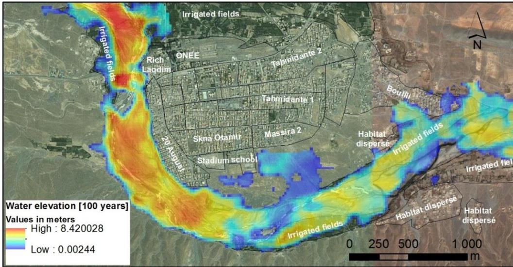
**Figure 8:** Centennial flood simulation (100 years)
